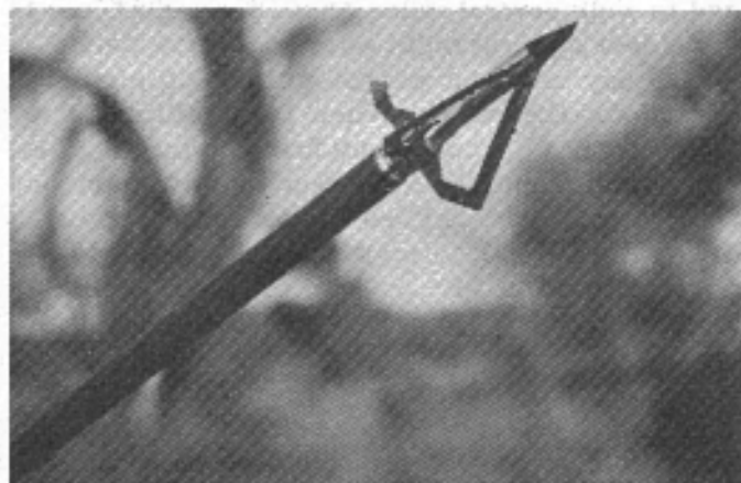
Typical result with an "Anderson 245" which stopped after hitting a rib on entry.
