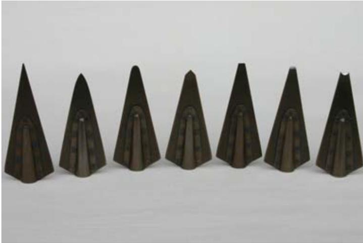
Tip designs tested included, from left: original needle-tip; COI arch-tip; COI round-tip; COI Tanto-tip; flat-tip; COI chisel-tip (flat); and COI concave-tip.
