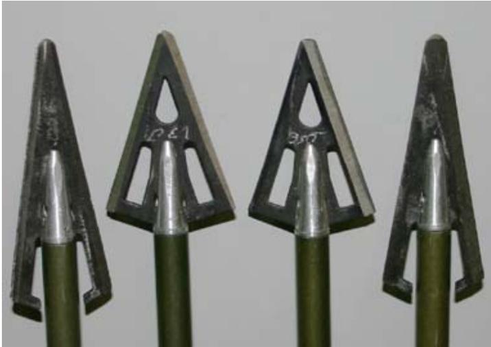
Narrow and wide-cut Outback broadheads tested. Left to right: narrow-cut double bevel (left); wide-cut double-bevel; wide-cut right-hand single-bevel; narrow-cut right-hand single-bevel. Not shown are the left-hand single-bevel heads tested. They would be the same as two single-bevel heads shown; merely with the bevel on the opposite edge of the broadhead.
