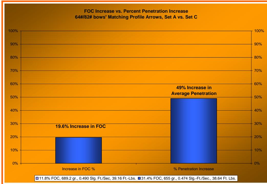
Graph 33 is a comparison between Sets A and C. Here we find that the 19.6% increase in FOC yielded an increase in average penetration of 49%.
