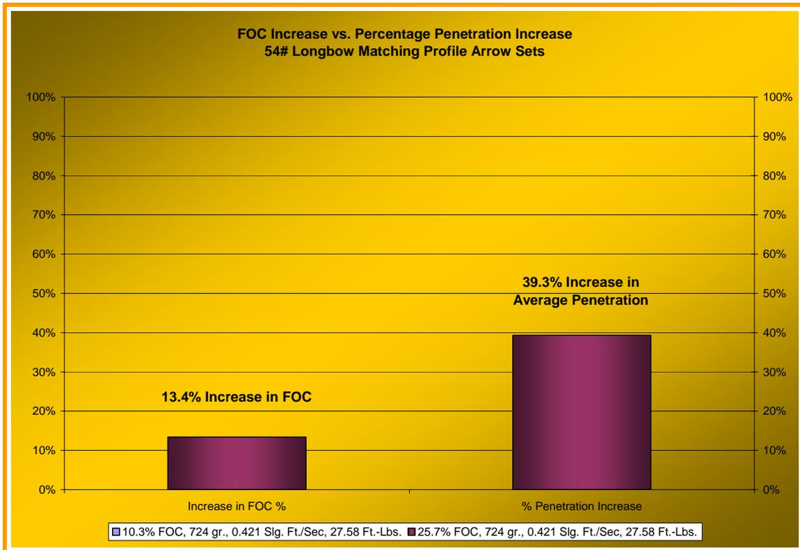
The arrow sets in Graph 28 are those tested from the 54# longbow. Specifics of the setup can be found in the 2007 Update, Part 4. The specifications pertinent for our purposes are: Set 1; 10.3% FOC, 724 grains, 0.421 Slug-Foot/Second of Momentum and 27.58 Foot-Pounds of Kinetic Energy (KE). Pertinent specifics for Set 2 are: 25.7% FOC, 724 grains, 0.421 Slug-Foot/Second of Momentum and 27.58 Foot-Pounds of KE.
