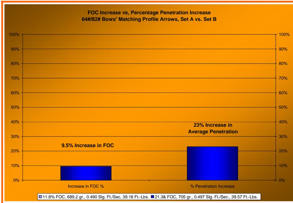
Graph 31 compares Set A against Set B. Both sets are fired from the 82# longbow. Here we find that a 9.5% increase in FOC resulted in an average penetration increase of 23%.
