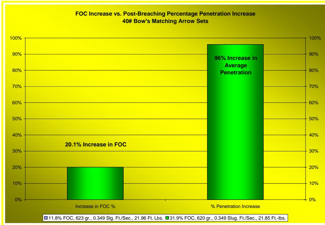
When we examine only the bone-breaching shots for the two sets of sub-threshold arrows from the 40# recurve (Graph 30) that same 20.1% increase in FOC shows an increase in average penetration of a whopping 96%.
