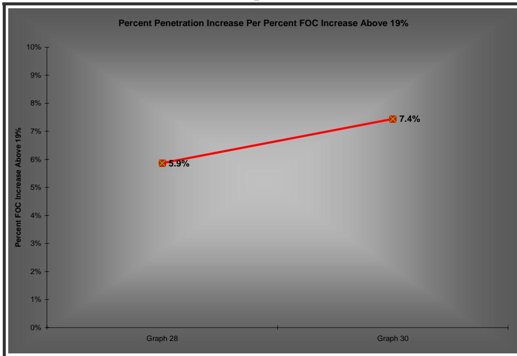
The red line in Graph 35 shows the average percent increase in penetration for every 1% the arrow's FOC was increased above 19%. This analysis for Graph 28's data indicates an average 5.9% increase in penetration for every 1% FOC was increased above 19%. Graph 29's analysis indicates an average of 7.4% increase in penetration per 1% increase in FOC above 19%. This implies that, above 19%, the *rate of penetration gain* is progressively increasing as the degree of arrow FOC is increased.
