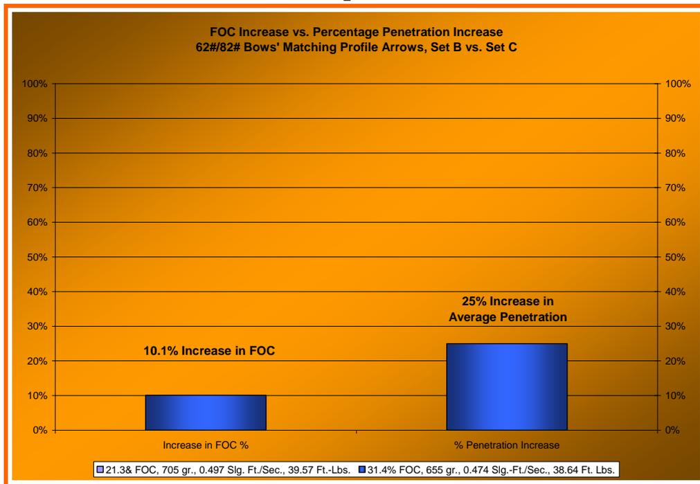
Graph 32 compares Sets B and C. In this comparison a 10.1% increase in FOC resulted in a 25% increase in average penetration.
