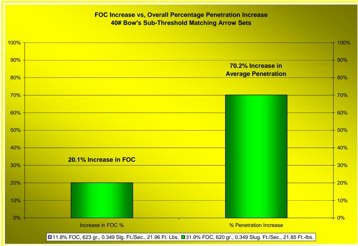
Graph 29 shows the similar FOC-to-penetration relationship for the sub-Heavy Bone Threshold mass Normal FOC and Ultra-EFOC arrows tested from the 40# recurve. The setup specifics are contained in Part 1 of on the current Update series. The pertinent specifications for each set are: Set 1; 11.8% FOC, 623 grains, 0.349 Slug-Foot/Second of Momentum and 21.96 Foot-Pounds of KE. Set 2: 31.9% FOC, 620 grains, 0.349 Slug-Foot/Second of Momentum and 21.85 Foot-Pounds of KE.
