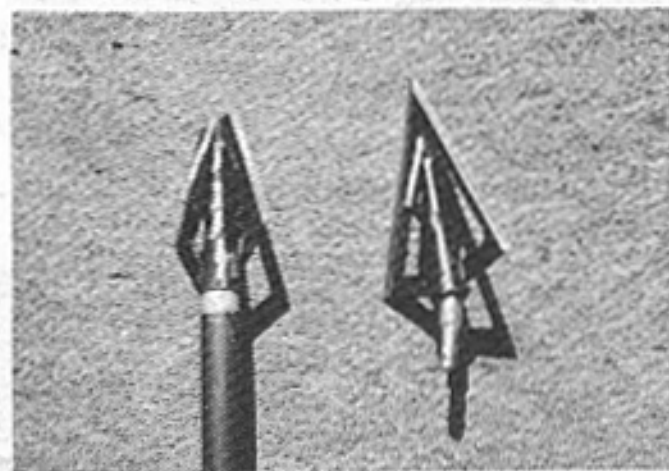
Shattered "Magnum II" broadhead that hit only soft tissue (L). "Magnum I" (R) notice bent adaptor.
