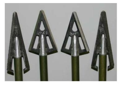
Narrow and wide-cut Outback broadheads tested. Left to right: narrow-cut double bevel (left); wide-cut double-bevel; widecut right-hand single-bevel; narrow-cut right-hand singlebevel. Not show are the left-hand single-bevel heads tested. They would be the same as two single-bevel heads shown; merely with the bevel on the opposite edge of the broadhead.
